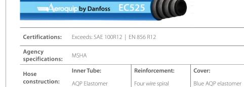
Typical fluids: -40°C To +149°C (-40°F To +300°F) Operating Phosphate-ester base fluids: -40°C To +82°C (-40°F To +180°F) temperature: Qualified 4S (-12 to -32) fittings:
